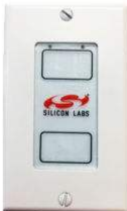
Figure 1.1. Zigbee Capacitive Sense Dimmer Switch Reference Design
