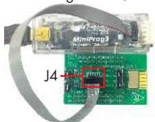
Fig 3: Programming/Debugging with MiniProg3
