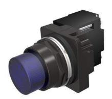
30mm BlackMax, Epoxy Coated Corrosion Resistant Complete Metal Unit Illuminated Indicator Light Transformer type, 120V AC Incandescent Lamp, BA9s Plastic Lens, Blue UL Listed, CSA Certified NEMA 1,3,3R,4,4X,12,13 & Automotive Standards
