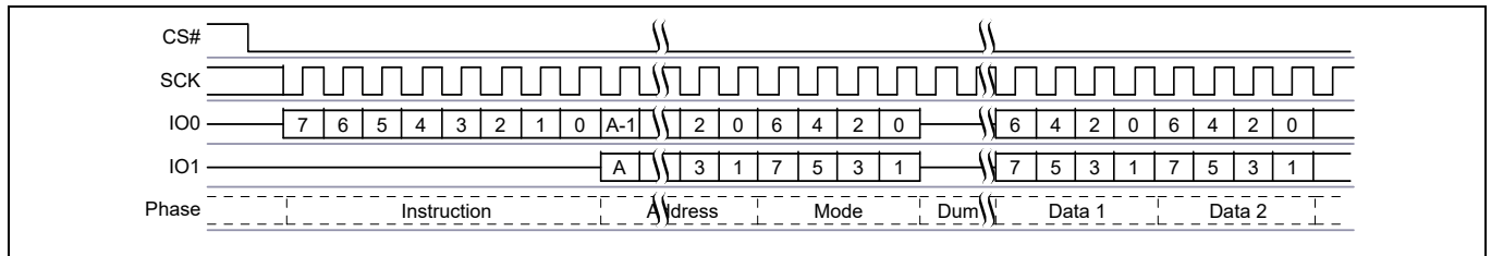
Figure 69 Dual I/O Read command sequence [32, 33]
