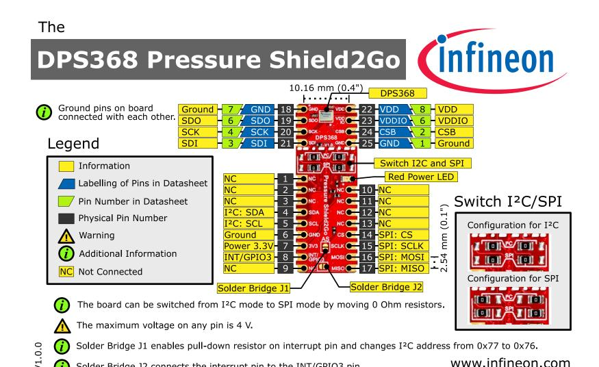
Solder Bridge J2 connects the interrupt pin to the INT/GPIO3 pin.
