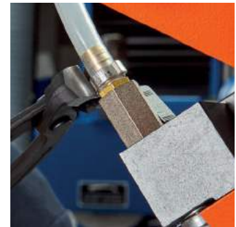
Sealing the hose connection on central lubrication
