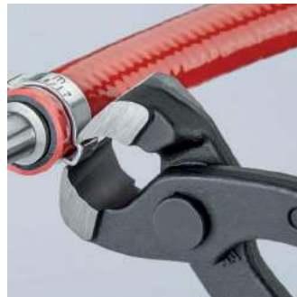
Sealing the fluid hose on the connecting piece
