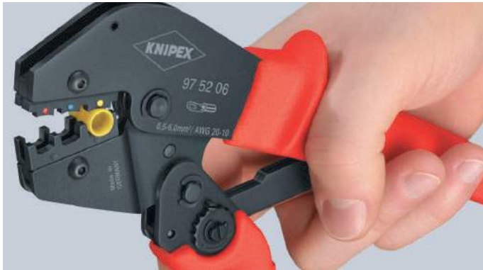
First step: place the connector into the correct crimping position. Squeeze handles slightly to secure connector inside die
