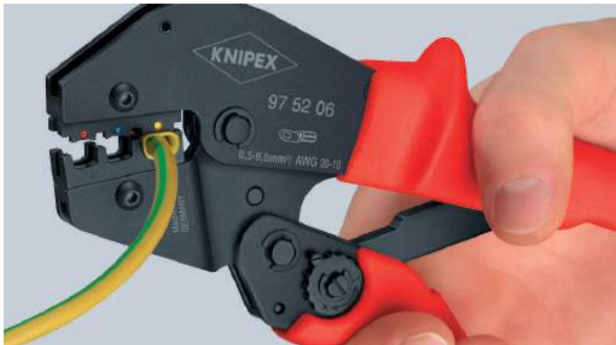
Second step: insert wire into connector and squeeze handles to complete crimp
