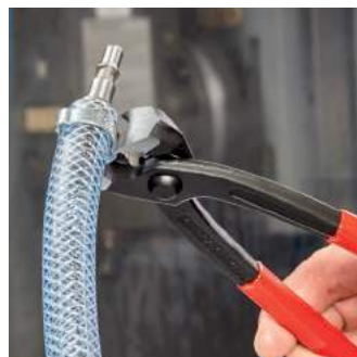
Sealing the pneumatic hose on the quick action coupling using the side press jaw
