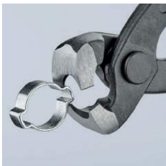
Using the front press jaw
