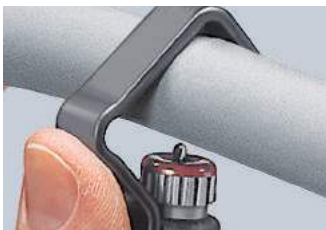
Setting the tool for circular cutting
