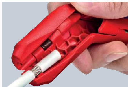
Stripping coax cable sheath
