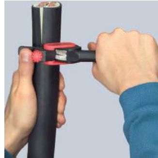
Turning the tool for circumferential cut
