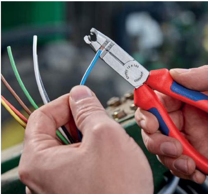
Wire stripping holes for 1.5 and 2.5 mm 2 conductors
