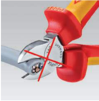
Cut performed with a Diagonal Cutter: high effort required, inaccurate cut, considerable deforming and crushing of the cable.
