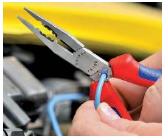
Crimping 20-14 AWG (0.5 to 2.5 mm 2 )
