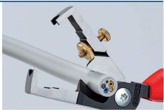
Induction hardened shear blade with precisely ground cutting edges for crushing-free cutting of copper cables up to 9/16" (15 mm Ø) (5 x 2.5 mm 2 )
