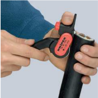
Setting the tool for longitudinal cut
