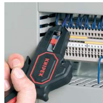
Stripping in confined areas
