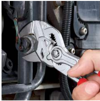
Working on plated fittings without damaging the surface
