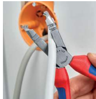
Cutting cable up to Ø 13 mm
