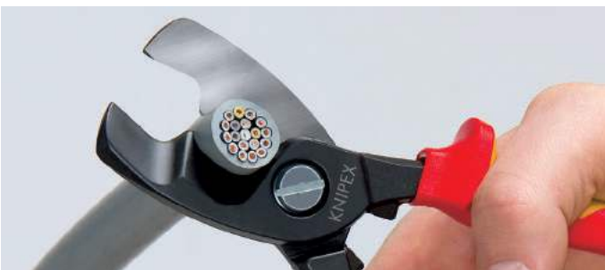
Final cut: after cutting the sheath in the front profile the conductors are cut in the rear area.
