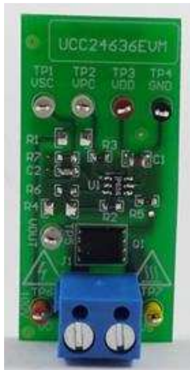
Figure 1. Photograph of EVM (Top Side)
