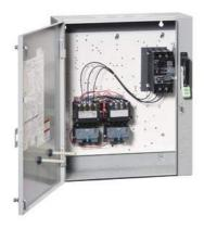
2-speed 3-phase motor starter, Size 1, Two separate windings, Constant horsepower, Solid-state overload relays, Low Spd OLR range 5.5-22A, High Spd OLR range 5.5-22A, 110V 50Hz / 120V 60Hz coil, Combination type, 25A circuit breaker, Enclosure NEMA type 1, Indoor general purpose use
