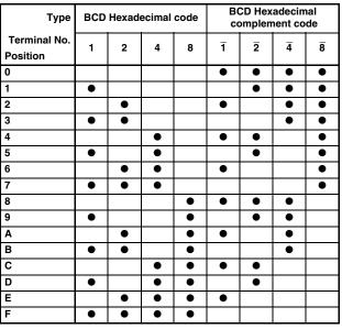
Note: "•" indicates that the internal switch is ON.
