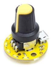
The Dial module is... a dial! It has a rotary potentiometer and five bright white LEDs that illuminate as the dial is turned.
