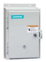
Non-reversing motor starter, Size 1, Three phase full voltage, Solid-state overload relay, OLRelay amp range 0.25-1a, 190 220/220 240V 50/60HZ coil, Non-combination type, Enclosure type 12, Dust/drip proof for indoors, Extra-wide enclosure
