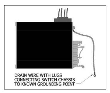
that there is no voltage difference between the power supply's negative output terminal and the chassis grounding point of the switch.
