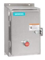
Non-reversing motor starter Size 2 Three phase full voltage Solid-state overload relay OLRelay amp range 13-52a 208VAC 60HZ coil Combination type Water/dust tight non-corrosive
