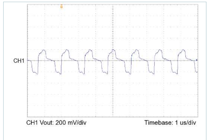
Figure 19 — Output voltage ripple, V_{IN} = 30\text{ V} , V_{OUT} = 12.0\text{ V} , C_{OUT\_EXT} = 1000\text{ }\mu\text{F} , R_{LOAD} = 0.896\text{ }\Omega
