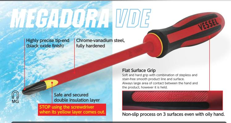
Commonly available screwdrivers with a shank cover is for the purpose of short-circuit prevention, NOT for electric shock prevention. The VDE mark is allowed to be on a product which has passed the 1000V energization test (all pieces).
