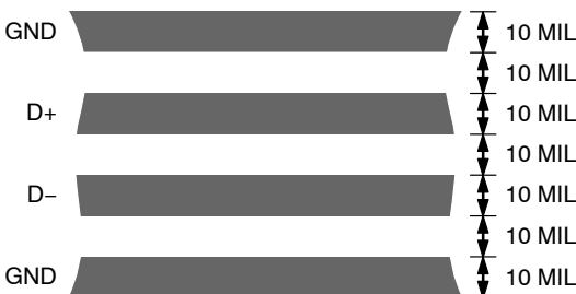
Figure 19. Arrangement of Signal Tracks
