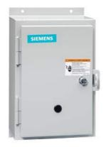
Non-reversing NEMA contactor, Size 1, Three phase full voltage, Contactor amp rating 27A, 3 wire (NO aux included), 110V 50Hz / 120V 60Hz coil, Non-combination type, Enclosure NEMA type 12, Dust/drip proof for indoors, Extra-wide enclosure
