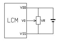
$V_{\text{DD}} \sim V_0$ : LCD Driving voltage
