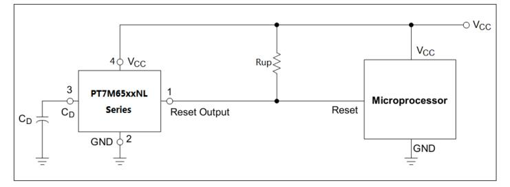
Note: Capacitor-Adjustable Delay application.
