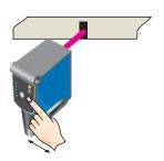
When setting the contrasts to be detected, the first LED (green) flashes in the bar graph.
