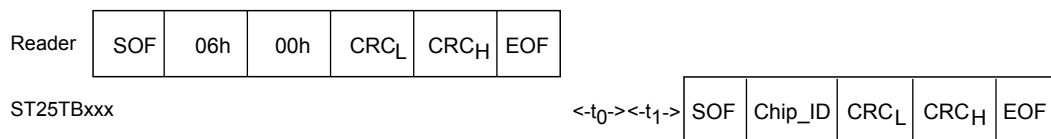
Figure 20. Initiate frame exchange between reader and ST25TB512-AC
