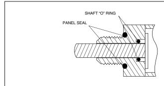
The shaft is sealed by an O-ring inside the bushing. The panel is sealed by an O-ring at the base of the bushing.
