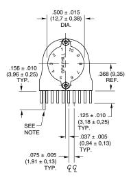
Note: Common location for a single pole per deck switch. For common location on two pole switches see circuit diagrams.
