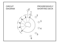
3, terminals 1,2, and 3 are connected to the common. Aprogressively shorting deck is limited to a maximum of 6 positions. A progressively shorting deck will function for 25,000 mechanical cycles of operation.
