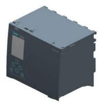
SIMATIC S7-1500F, CPU 1518F-4 PN/DP MFP, central processing unit with C/C++ Runtime pre-installed, 9 MB work memory for program and 60 MB for data, 1st interface: PROFINET IRT with 2-port switch, 2nd interface: PROFINET RT, 3rd interface: Ethernet, 4th interface: PROFIBUS, 1 ns bit performance, SIMATIC Memory Card required
