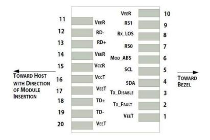
Pin-out of connector Block on Host board
