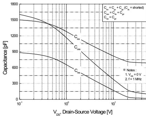
Figure 5. Capacitance Characteristics
