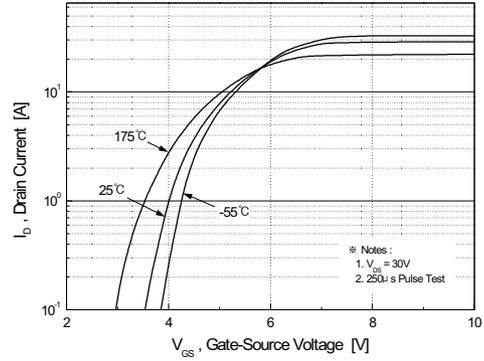
Figure 2. Transfer Characteristics
