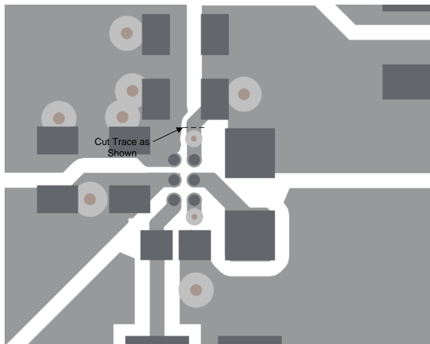
Figure 1. Loop Response Measurement Modification
