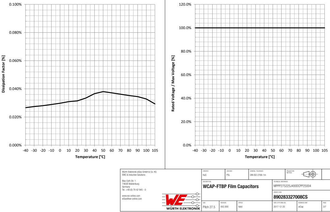
**Rated Voltage vs. Temperature:**
