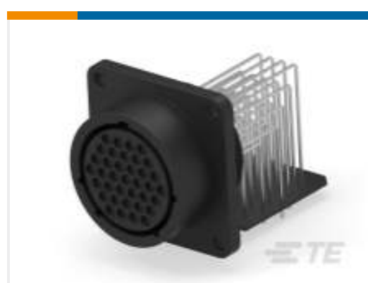
TE Part # 1-796409-1 CPC PSTD RCPT,23-37,R/A LF
