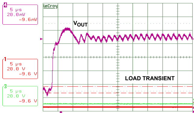
FIGURE 16. LOAD DUMP RESPONSE AT THE CPU SOCKET MPGA479, 35A LOAD STEP @ 200A/μs, 2 PHASE CCM
