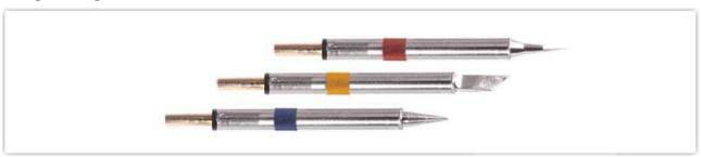
1 Easy Braid Co. tip cartridges will typically idle within a temperature range of +/-1.1°C. However, there is variation in idle temperature across tip geometries within an individual temperature series. Easy Braid Co. offers a wide variety of tip geometries from 0.25mm fine point tip to 5mm chisel. The length and geometry of a tip will have an influence on the tip idle temperature. To accurately measure idle temperature it will depend greatly on the measurement method,
