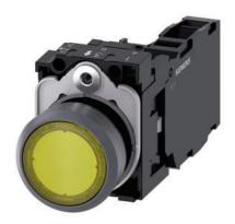
Illuminated pushbutton, 22 mm, round, plastic with metal front ring, yellow, pushbutton, flat, momentary contact type, with holder, 1 NO+1 NC, LED module with integrated LED 24 V AC/DC, screw terminal
