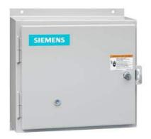
Non-reversing motor starter, Size 1, Three phase full voltage, Solid-state overload relay, OLR amp range 0.75-3.4A, Non-combination type, Enclosure type 12, Dust/drip proof for indoors, Standard width enclosure
