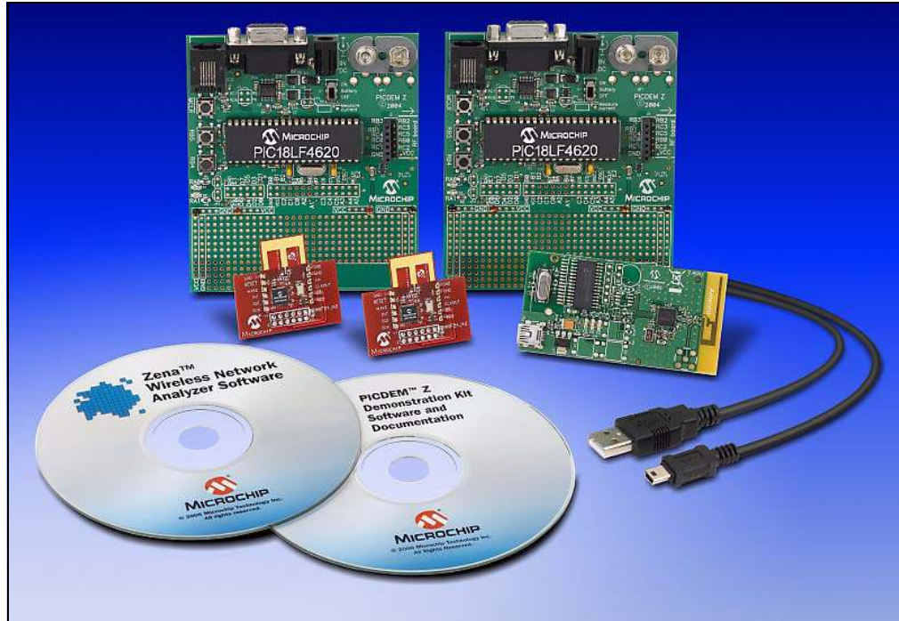
FIGURE 1-1: PICDEM™ Z DEMONSTRATION KIT
