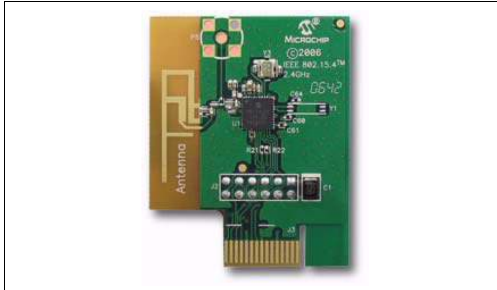
FIGURE C-1: PICDEM™ Z MRF24J40 2.4 GHZ DAUGHTER CARD
