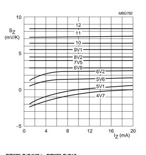
Fig.6 Temperature coefficient as a function of working current; typical values.
