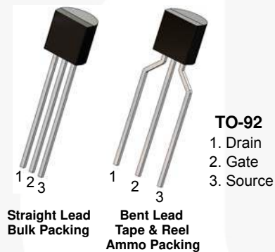
Figure 1. J175 / J176 Device Package
