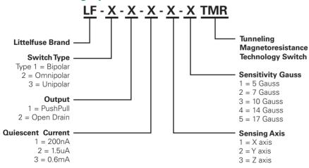
Example: LF21215TMR is an Omnipolar, PushPull, 1.5uA, X axis, 17 Gauss Note: Every combination is NOT offered. Contact Littelfuse for availability.
