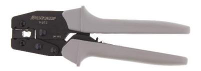
Crimping tool for crimping wire-end ferrules with and without plastic collars. Cross-section range: 50 mm². Easy to use, Auto-lock for proper and complete crimping, Wire can be fed in from the side, Self-opening with built-in spring.
