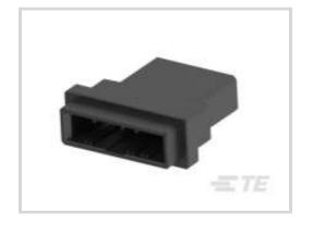
Connector Product Type: Housing Connector & Housing Type: Housing for Male Terminals Connector System: Wire-to-Wire Number of Positions: 5 Centerline (Pitch): 3.81 mm [.15 in ]
