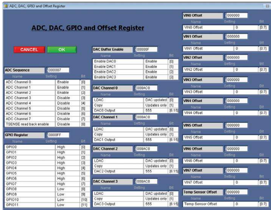
Figure 25. ADC, DAC, GPIO, and Offset Register Window
