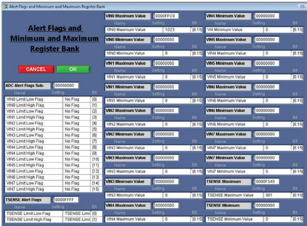
Figure 27. Alert Flags and Minimum and Maximum Register Bank Window
