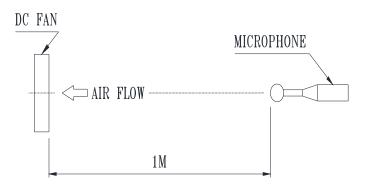
NOISE IS MEASURED AT RATED VOLTAGE IN FREE AIR IN SEMI-ANECHOIC CHAMBER WITH MICROPHONE AT A DISTANCE OF ONE METER FROM THE FAN INTAKE.
