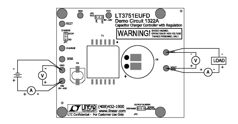
Figure 1. Proper Measurement Equipment Setup
