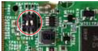
Figure 2: SW602 setting for Serial Download Mode
