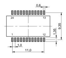
no vias or traces underneath the component Scale - 2,5:1
