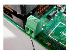
STK502 supports both the In-System Programming mode and the High-voltage Programming mode. AVR Studio, Atmel's front-end tool for the STK500 Development Board, provides support for STK502.
