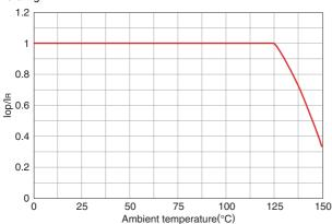
Maximum current value for the ambient temperature (mA) Ambient temperature Part No
