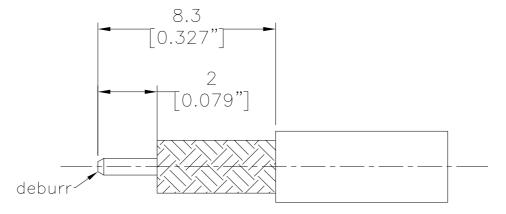
RECOMMENDED CABLE STRIPPING DIM'S Connector Adds: 10.7 mm
