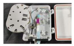
15. Feed the patch cables into the bottom of the grommet. Reinstall the grommet into the bottom of the distribution box. Make sure each strand of the patch cables fit in a single spot within the cable clamp area.
