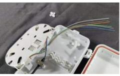
11. Lay the fiber ends between the edge of the distribution box and the base of the cable "T" under the splice tray, then reinstall the "T" top. Terminate the fibers as needed.
