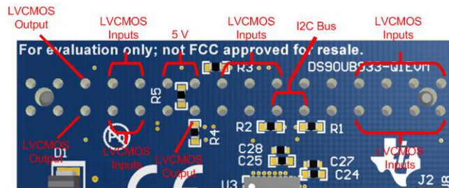
Figure 4. Parallel Input Connector on Serializer Board
