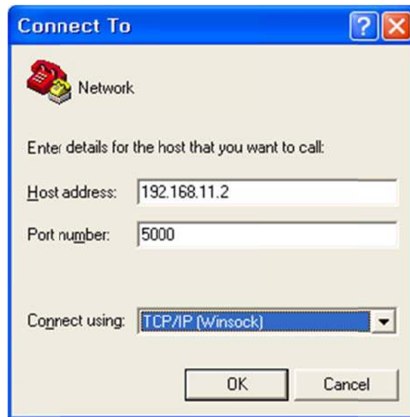
Figure 18. Network Terminal Program configuration
