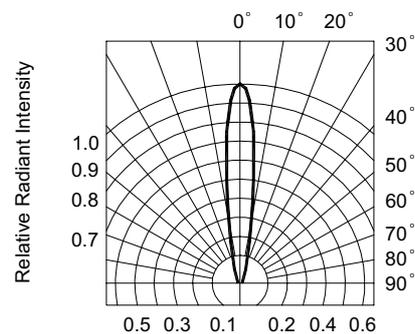
FIG.6 RADIATION DIAGRAM
